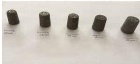
**Fig. 1.** Set of subtalar porous titanium nickeline implants
